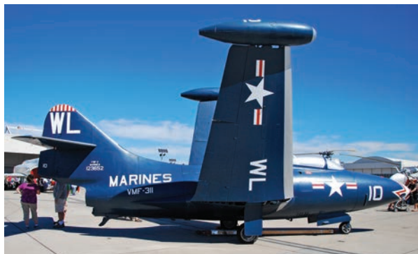
F9F-2 First production version, powered by Pratt & Whitney J42 engine. Marine Corps Air Station Miramar (MCAS Miramar) (IATA: NKX, ICAO: KNXX, FAA LID: NKKX) Photo: Tomás Del Coro Miramar Air Show 2014 October 4, 2014
